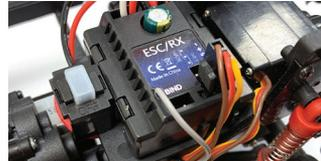
The ESC/receiver switch is located under the bodyshell of the model. Switch on the ESC/receiver switch shown here.
